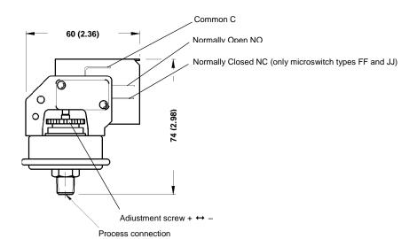
Fig. 11: Diaphragm seal piston pressure switch type MSPS-...
