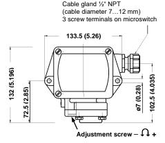
Diaphragm seal piston pressure switch type P1H-...
