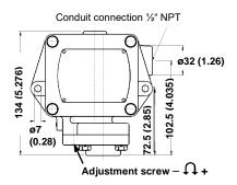
Fig. 10: Diaphragm seal piston pressure switch type P1X-...
