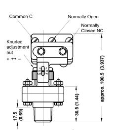
66.5 ±0.5 (2.62 ±0.02) Cable gland M20×1.5 (cable diameter 7...12 mm) 34 (1.34) max. 85 (3.346)
