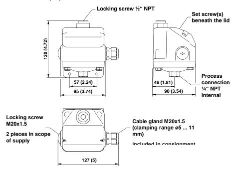
Fig. 7: Metal-diaphragm pressure switch type D1T .../D2T ...
