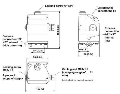
Fig. 8 Metal-diaphragm differential pressure switch type DPD1T .../DPD2T ...
