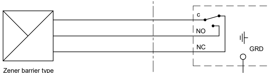
Fig. 6: Operation of pressure switches in intrinsically safe areas
