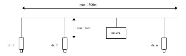
The following RS485 driver is used in the devices: MAX3471
