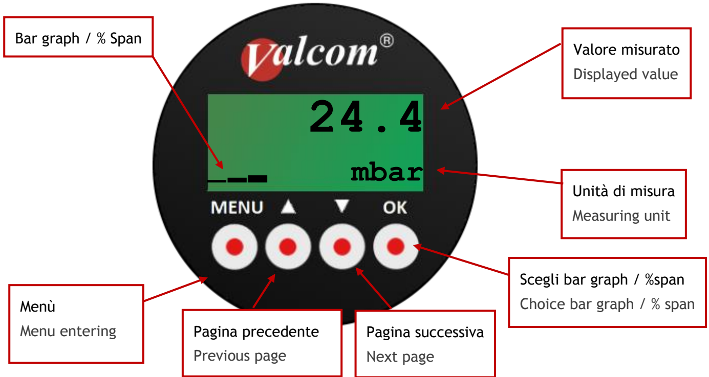
Figura / Figure 11 : Display LCD e tastiera / LCD display and keyboard
